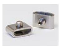
Screwbinder™ Buckles are used in applications when a temporary clamp is desired or space limitations do not allow a tool roll-over. A set screw locks the band after tensioning.
